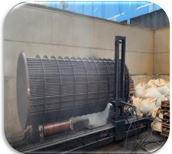
Bundle Outside Cleaning
